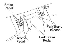
pedal returns normally before starting the engine. Make sure there's adequate throttle pedal freeplay. See page 86 for throttle pedal adjustment procedures.
